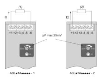
(1):  $R_{Load1}$ (2):  $R_{Load2}$  $R_{Load1} = R_{Load2}$  $I_1 = I_2 = -I_{nom}$
